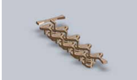
Figure 1. Design of a SAR PSM micromixer
