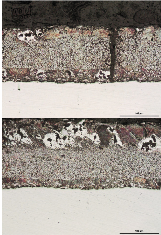
Fig. 2. Zn - Al 5 wt% bath microstructure (two different points on coating section).
