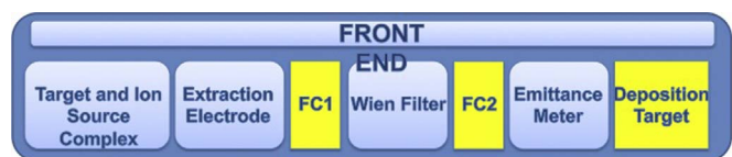
Fig. 5. Schematic representation of the Front End off-line with its main components. FC1 and FC2 are the two Faraday Cups, diagnostic devices, placed before and after the Mass Separation system (the Wien Filter).
