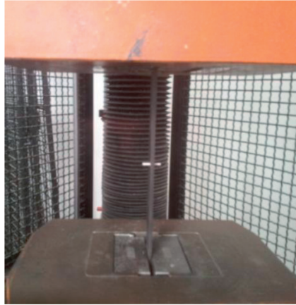
Fig. 4. Lateral view of the coupon with pin in the Test Machine, FHT
