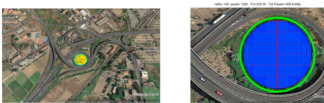
Figure 9. Catania airport Junction. Diameter 75 m power 400 kWp.
