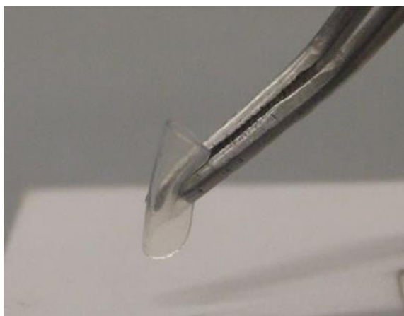
Fig. 9. Picture of manually folded Ss-PS lens.
