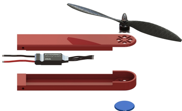
Figure 8: Electronic and avionic elements in the arm for the single rotor configurations.
