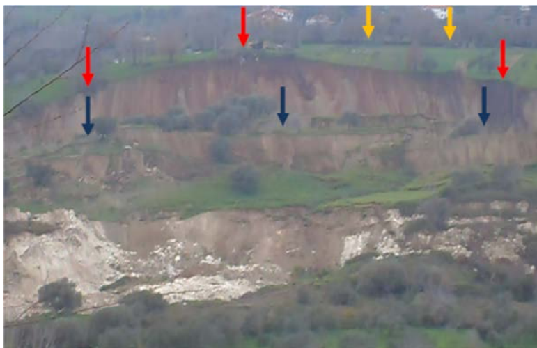
Fig. 3. The 15 February 2010 landslide with an indication of the main slip surface at 300 m elevation (red arrows) and a second slip surface emerging at 285 m elevation (blue arrows). The pre-existing scarp at 305 m a.s.l. (yellow arrows) was not involved by the failure process.
