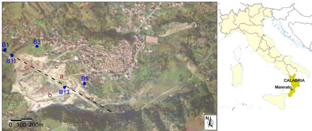
Fig. 1. Aerial view of the 15 February 2010 Maierato landslide and location of the Maierato village (Calabria, Southern Italy). Legend: a, b and c location of the photos in Fig. 2; B1, B3, B5, B11 and B13 location of the boreholes in Fig. 6; ----- trace of section.
