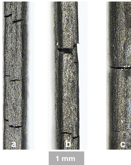
Fig. 9. Light Optical Microscope observation of the hydrogen charged 2101 DSS (three different heat treatments: a) rolled; b) 450°C 3-h; c) 600°C-3h).
