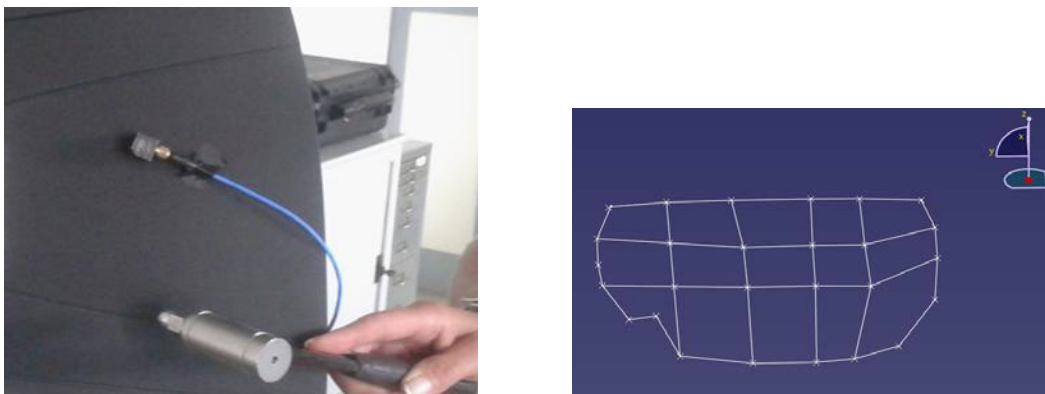
Fig. 5. Test set up and equipment (left); geometry structure (wireframe) used for modal impact test (right)
