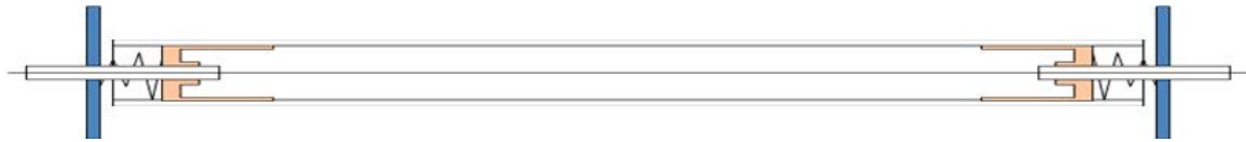
(a) Schematic cross-section of a single straw tube.
