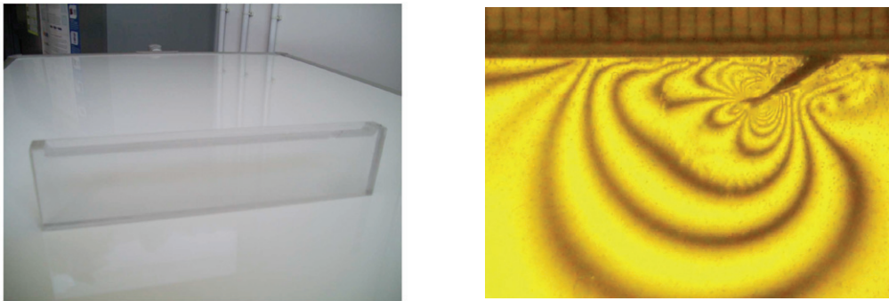
Figure 3: Uncracked sandwich (left); photo elastic results for dry model (right).
