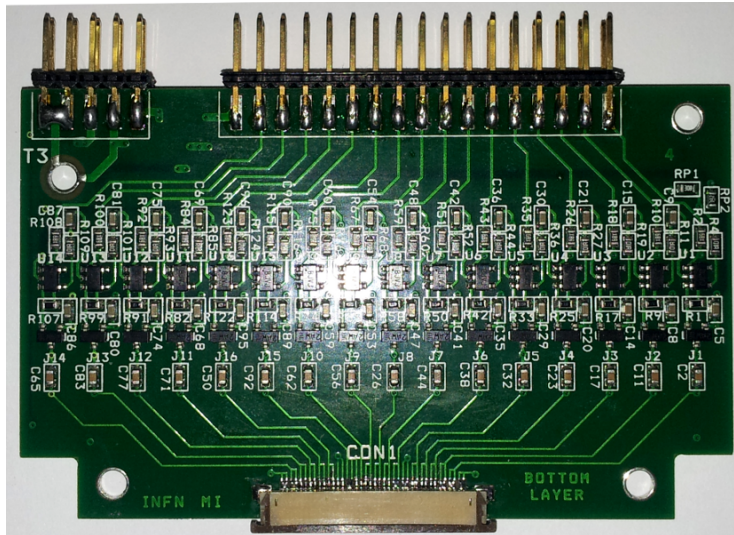
Figure 9. (color online) PCB housing 16 charge-sensitive preamplifiers for the electronic readout of signals originating from one side of the 40/60 \mu\text{m} -thick DSSSD detector (16 channels/side). The ERNI 36-pin connector, where the input Kapton cable is inserted into the PCB, is located on the PCB bottom part. The board power supply connector (left) and the output signal connector (center) are placed on the PCB upper part.
