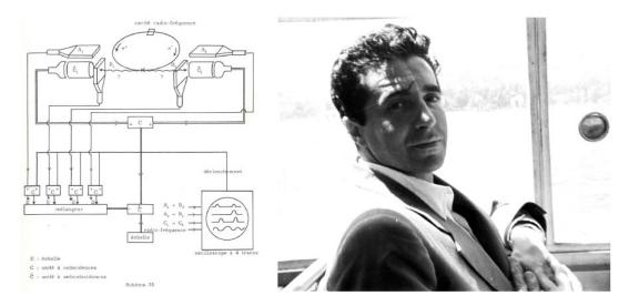
Figure 21: The logical scheme for measuring the process  $electron + positron \rightarrow 2\gamma$ , from Jacques Haïssinski's thesis. The  $\gamma$  rays exiting AdA (center top) are depicted as two wavy lines labelled  $\gamma$ , to be detected by an assembly of electronics and detectors. The apparatus, was constructed by Giuseppe Di Giugno and Ruggero Querzoli, who is shown here in the right panel.
