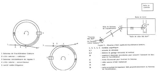
Figure 16: Figures 4 and 5 from from Jacques Haïssinski's thesis show the positioning of AdA with respect to the linear accelerator and the translating platform at right, with mechanism of injection of electrons and positrons, at left.
