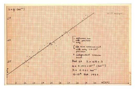
Figure 22: The linear correlation between the number of particles in one bunch and the inverse of the lifetime, at the nominal AdA energy, in a plot by Touschek's own handwriting (Original document in Carlo Bernardini, personal papers). The data were reproduced in Fig. 1 of (Bernardini *et al.* 1964).
