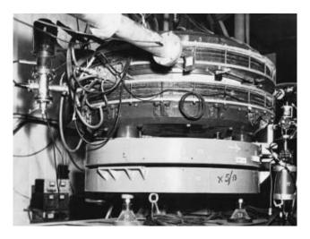
Figure 17: AdA on the rotating and translating platform at Orsay. On the left the injector beam channel. Courtesy of Jacques Haïssinski.
