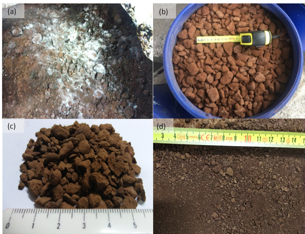
Fig. 2. Lignin B (a) as received, as used in the updraft gasification test (b), as used in the BFB gasification test (c) and as used in the indirect gasification test (d).
