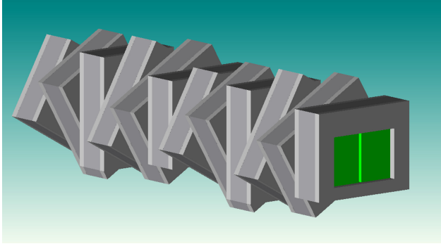
Fig. 2: Sketch of the collimation system layout. (This image was obtained directly from MCNPX input file, using MCAM by FDS team, China [13]).
