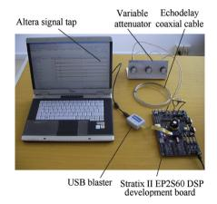
Fig. 4. Electrical test layout for the first LIDAR electronic prototype.
