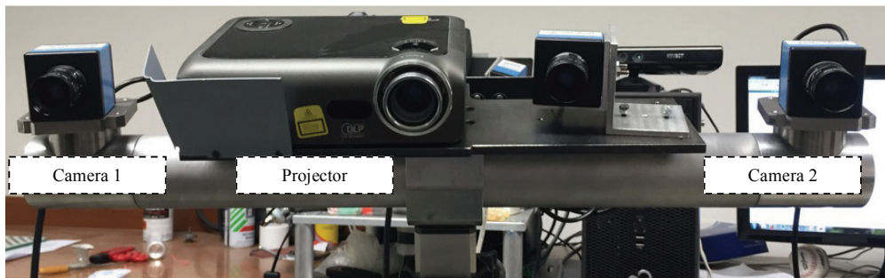
Fig. 2. 3D Optical scanner composed of two digital cameras and a multimedia projector.
