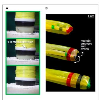
FIGURE 4 | Organism-inspired robots. (A) The first implementation of the growing robot inspired by plant roots, with a thermoplastic material used to build the structure with additive manufacturing (Sadeghi et al., 2017); (B) Body elongation sequence of the soft robot with skin eversion induced by pressurization (From Hawkes et al., 2017. Reprinted with permission from AAAS).
