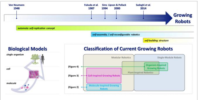
FIGURE 1 | Top: major milestones in relation to growing robots and the concepts developed from the most important contributions. Bottom-left: biological models used for the classification of growing robots. Bottom-right: robotic groups explored in the literature (modular and plant-inspired robotics).
