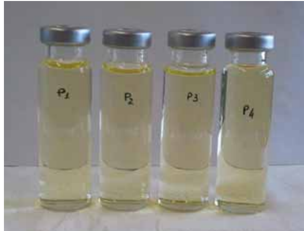
Fig. 3. Macroscopic aspect of \beta -C nanoparticles suspensions produced by SAILA with variation of GLR. Process conditions are reported in Table 1.
