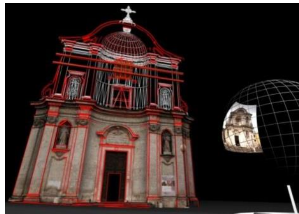
Figure 1. 3D model (low-poly) with photorealistic texture from oriented spherical panoramas
