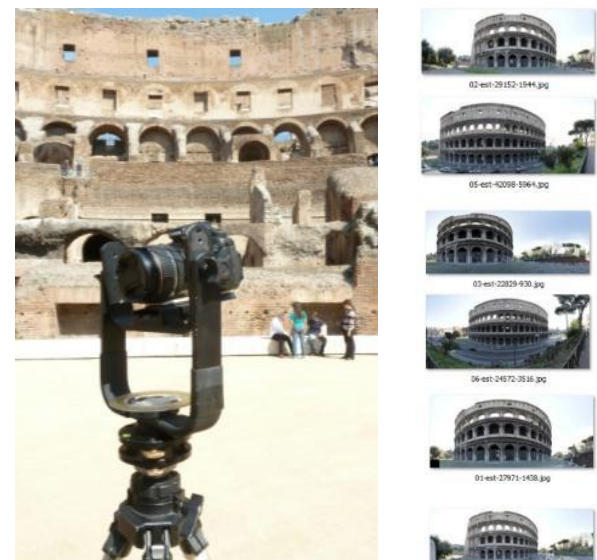
Figure 5. Acquisition instrument and panoramic photos
