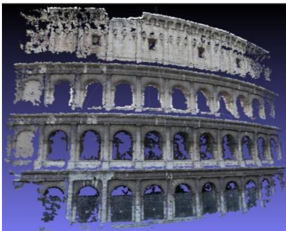
Figure 12. Automatic restitution of 3D points by SfM
