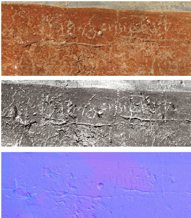
Figure 6. RTI outputs: Default mode (above); Specular Enhancement (middle); Normals Visualization (below)
