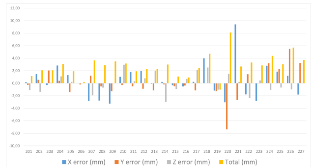
Figure 5. Ground Control Point errors of long wall photogrammetric set
