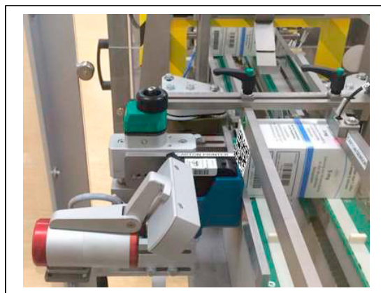
Fig. 5. Labelling phase of a unit box.
