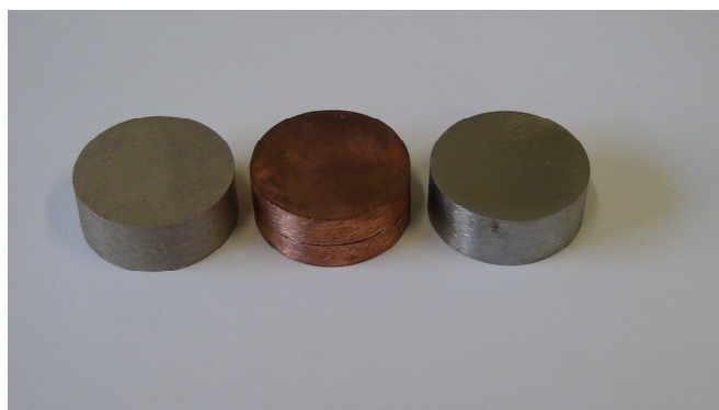
Figure 1. Picture of Ni-coated (left), Cu-coated (middle) and uncoated (right) samples
