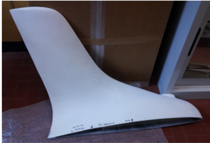
Fig. 1. The investigated composite full scale blended winglet
