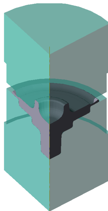
Fig. 2. The forged part inside the dies at the end of first forging blow.
