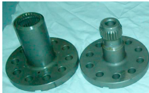
Fig. 3. spline coupling used for wear tests.
