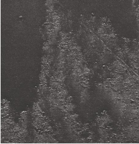
FIGURE 1: High-resolution synthetic aperture sonar image showing the acoustic backscatter from a patch of seabed measured with the MUSCLE system by NURC off the coast of Latvia. Range runs downward and along-track from left to right. The total image is 30 by 30 meters.
