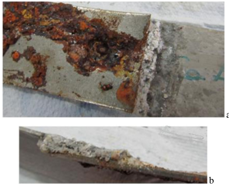
Figure 5 Al oxide layer in St1/Al1.5 (a) and in St1.5/Al1 (b).
