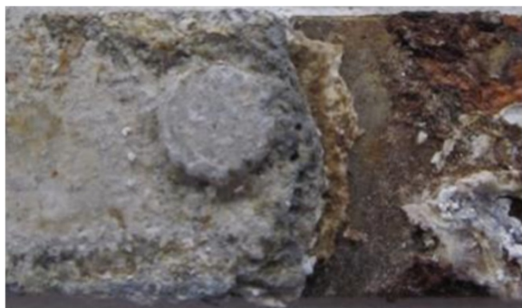
Figure 6 Progressive Al thinning in a St1/Al1.5 joint at 10 weeks.
