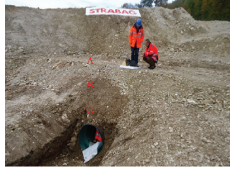
FIGURE 7: Test scenario: a victim is buried by 2 m of excavated ground.
