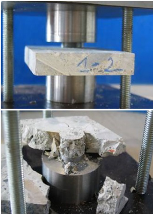
Fig. 11. Double Punch Test for mortar courses. It is easily detectable the formation of a central compressed kernel.
