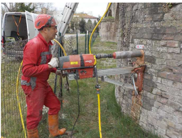
Fig. 16. Extraction of specimens from positions 4.
