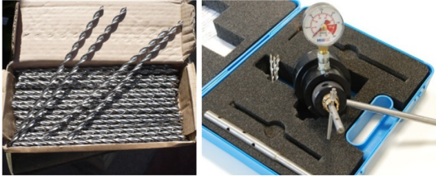
Fig. 4. Helical fasteners and Helifix pull out tester.
