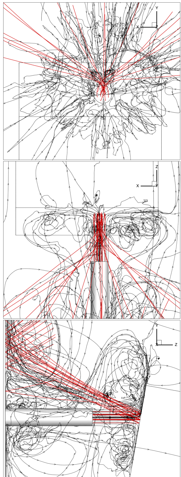
Fig. 12 Streamlines and cloud trajectories in the first evolution step
