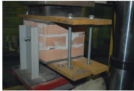
FIGURE 4: Sample 2a placed in the testing machine, before the application of the load.
