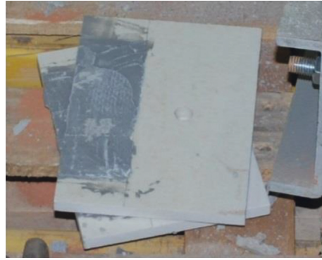
FIGURE 7: Shear failure of the adhesive in samples 1a-b.
