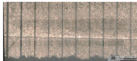
Fig. 4. Macrograph of the markings on the titanium cold sprayed layer performed at Pp=20 kW.
