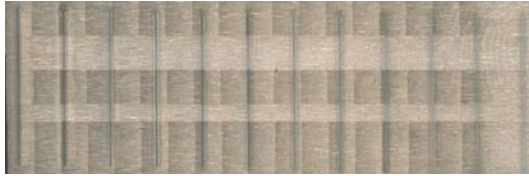
Fig. 5. Macrograph of the markings on the titanium sheet performed at Pp=20 kW.
