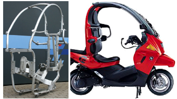
Fig. 5. Tubular frame structure of the BMW C1.
