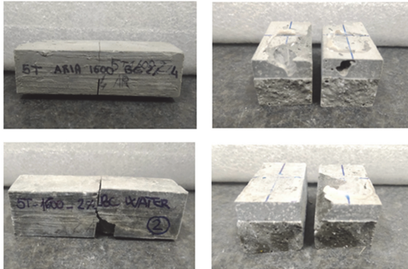
Figure 7: Fracture path and fracture surface of four analyzed foamed concrete notched beams with 2% biochar cured in air (top) and in water (bottom).
