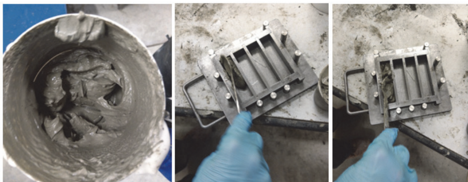
Figure 1: Foamed concrete paste at the fresh state (left) and pouring into formworks for the realization of prismatic beams.
