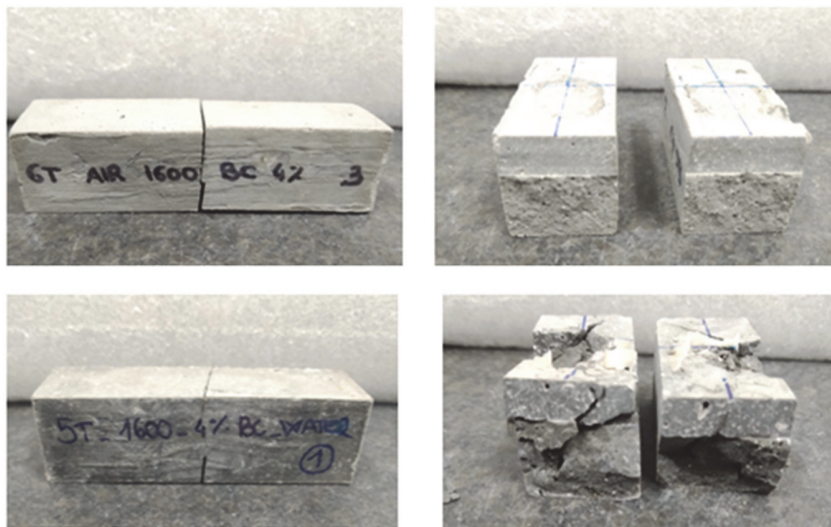
Figure 8: Fracture path and fracture surface of four analyzed foamed concrete notched beams with 4% biochar cured in air (top) and in water (bottom).
