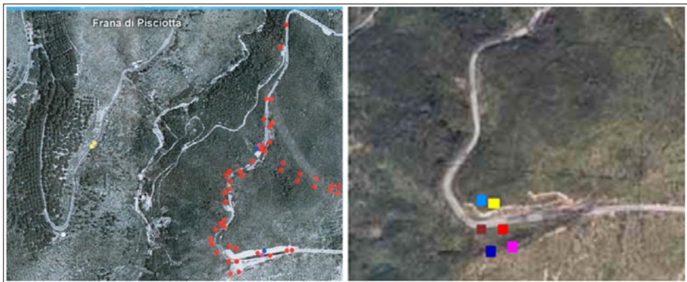
Figure 2 - Topographical monitoring by the Iside group: left panel: the control points location; the right panel: a few details about points P01÷P06 ( http://www.centroiside.net ).
