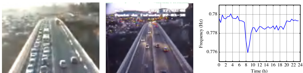
Fig. 3. From left to right: typical traffic in the periods from 7:00 to 10:00, and from 10:00 to 19:00; daily evolution of the first natural frequency.
