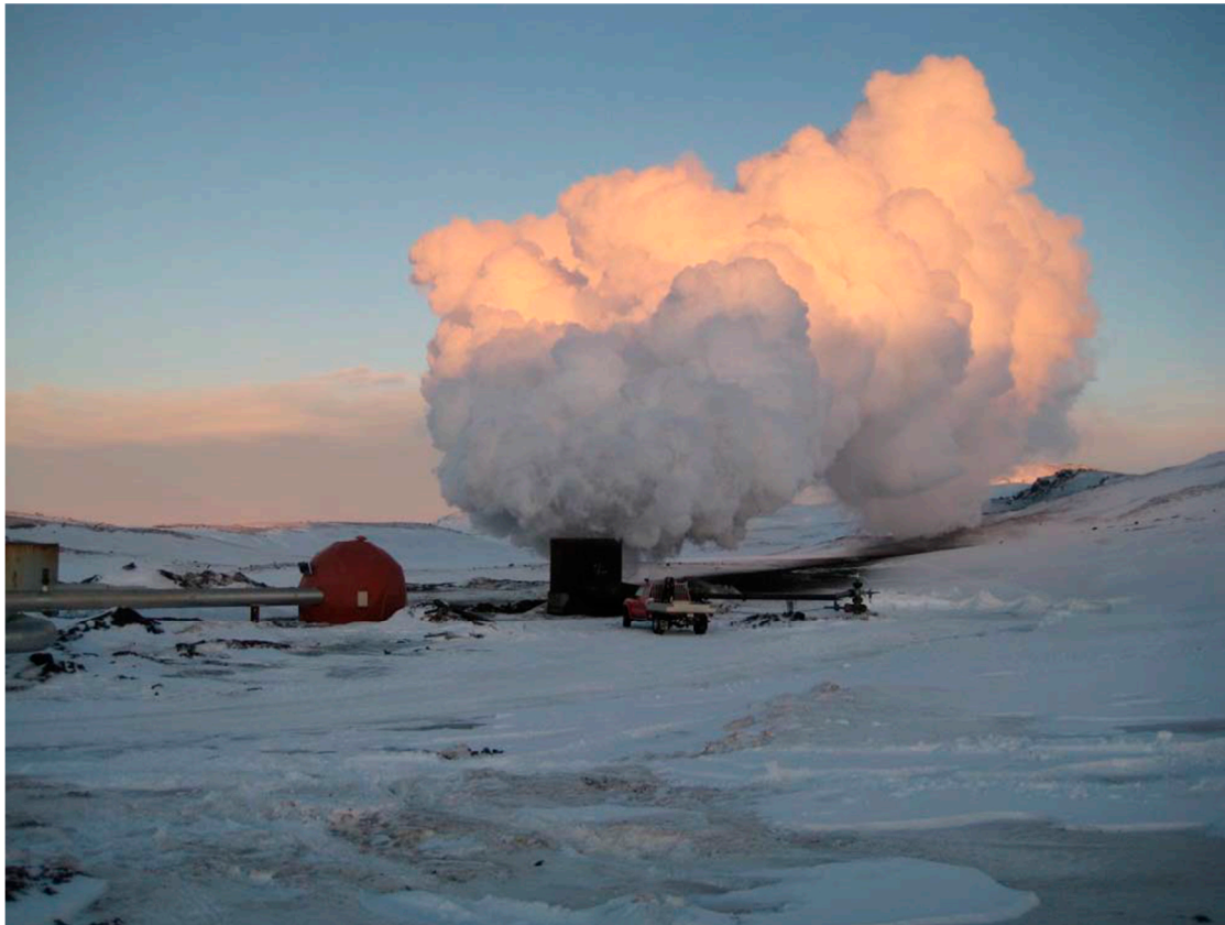
Figure 2. Flow test of Well KJ-36, Krafla Caldera, Iceland on 12 December 2007. Just two super-hot wells such as this near-magma borehole and IDDP-1, which penetrated rhyolite magma [14], could power Landsvirkjun’s 60 MWe power plant at Krafla, if the engineering challenges can be overcome. The well slants under Viti Crater (cover photo) and reaches a vertical depth of about 2500 m approximately 500 m north of the crater. Photo credit: Ásgrímur Gudmundsson.
