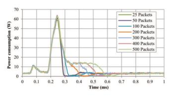
Fig. 1. Energy consumption of the CPU when receiving a burst of a variable number of packets.
