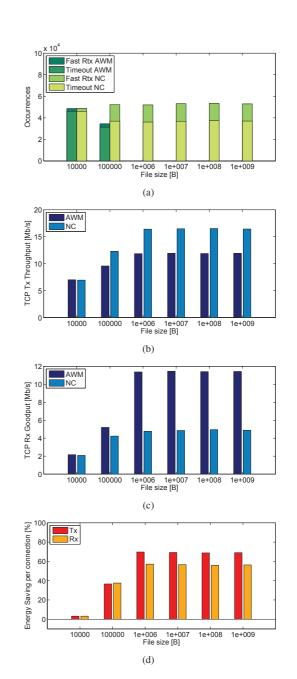
Fig. 4. Timeouts and Fast Retransmit occurrences (a), Transmitted Throughput (b), Received Goodput (c) and AWM Energy saving per Connection (d) when the network is loaded by greedy TCP traffic.
