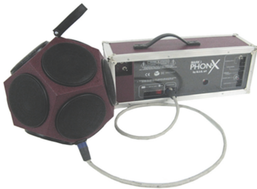
FIGURE 3: Dodecahedron FOUR and amplifier PHON-X Mark I.
