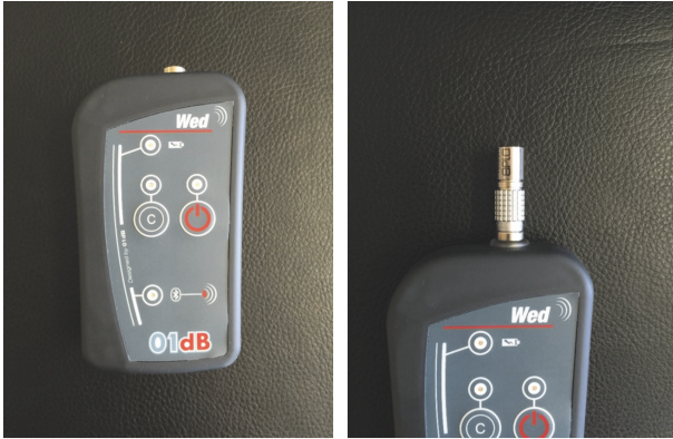
FIGURE 2: Noise dosimeter WED 007 with microphone, 01 dB.
