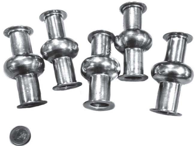
Figure 2. A set of 6 GHz Nb monocell cavities.
