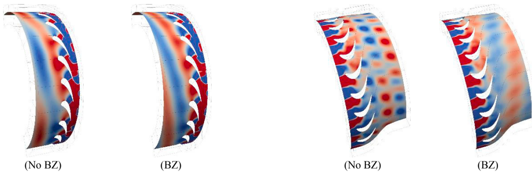
Fig. 4. Acoustic pressure perturbation at stator (left) and rotor (right) midspan section without and with buffer zone application.
