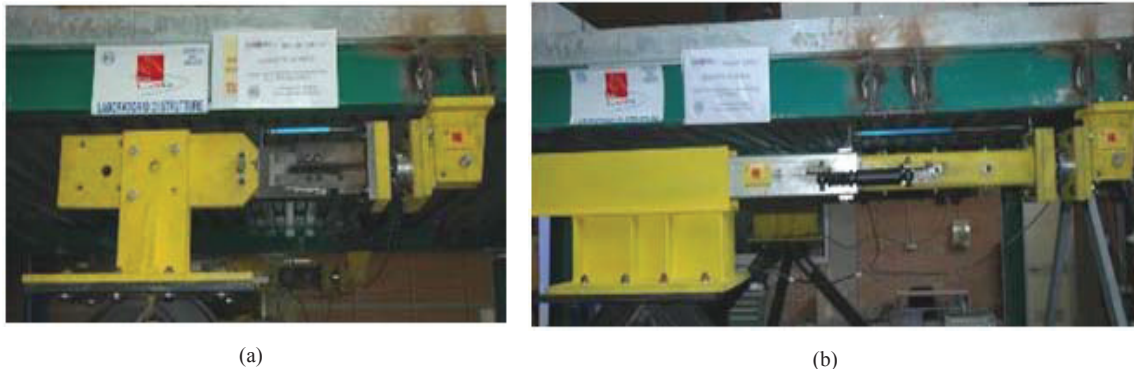
Figure 4: Dissipating devices considered in the experimental tests: a) HD and b) SMA+VD
