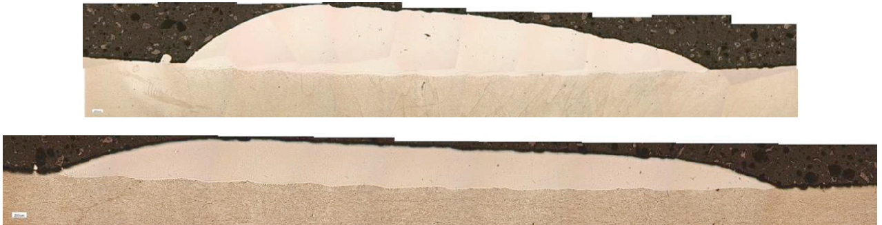
Fig. 4. Cross-section samples at high energy (sample above) and low energy (sample below).
