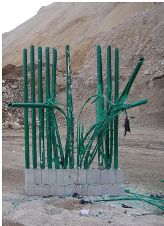
FIGURE 6: Barrier specimen after the third test.
