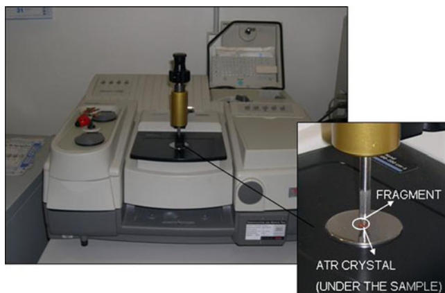
Fig. 1 ATR Smart Orbit™ mounted on a Thermo Nicolet Nexus 5700 spectrometer
