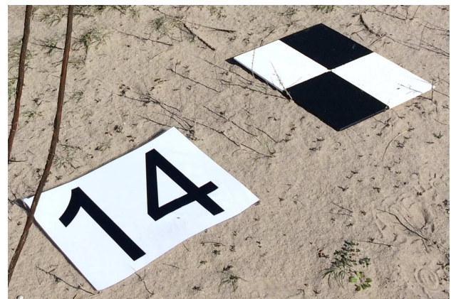
Figure 4. Example of a target used as Ground Control Point
