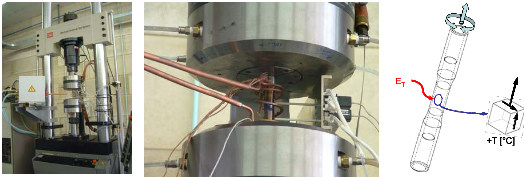
Fig. 3. Multi-axial (axial/torsional) fatigue testing equipment and applied strain.
