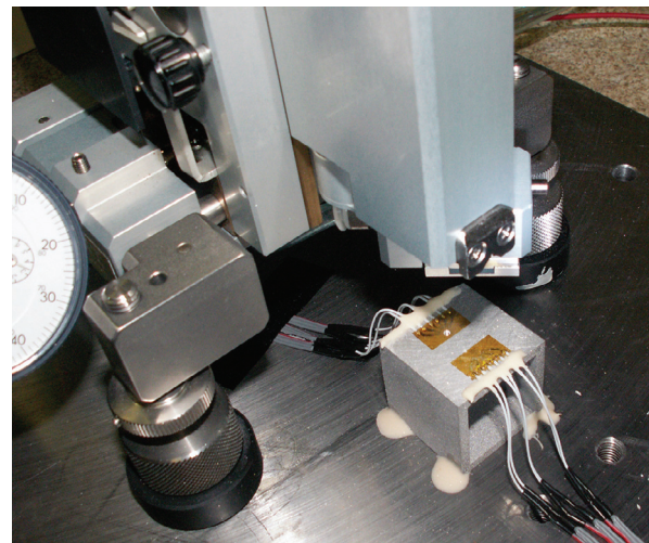
Fig. 3. MTS3000 RESTAN (REsidual STress ANalyzer) system by SINT Technology during a measurement phase on specimen E.
